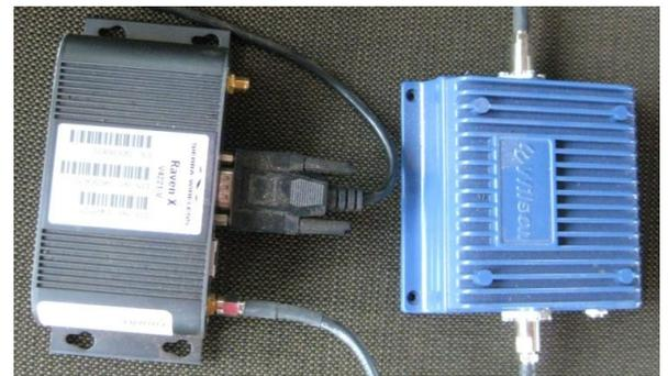
Figure 1. Example cellular modem (left) and optional cellular signal booster (right).
