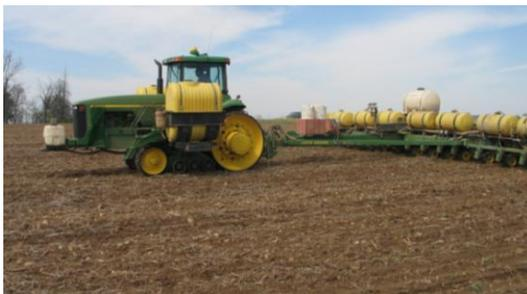
Figure 1. Example of a planter equipped with VRT.
