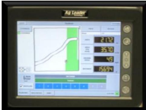
**Figure 2. Example screen capture from a display showing a coverage map when using Automatic Section Control technology on an 8-row planter.**
